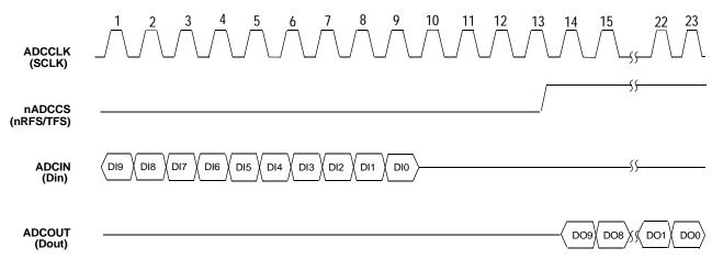
Figure 25. SSI Interface for AD7811/2
