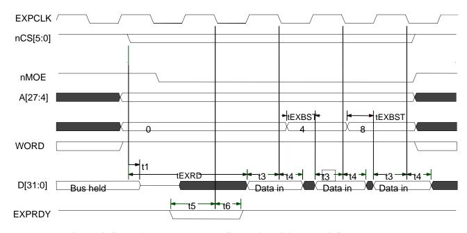
Figure 14. Sequential Page Mode Read Cycles with Minimum Wait States
