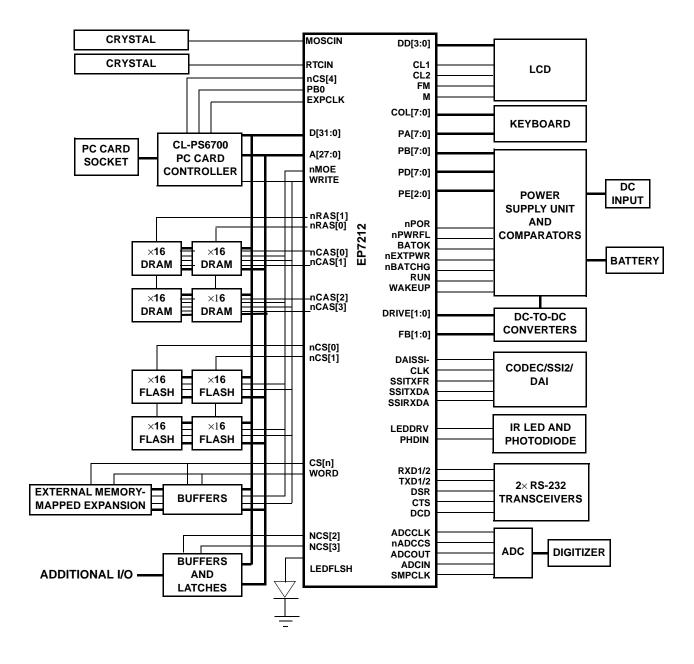
**NOTE:** A system can only use one of the following peripheral interfaces at any given time: SSI2, codec, or DAI.
