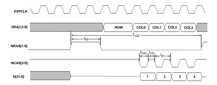
Figure 21. Quad Word Read from DRAM at 36 MHz
