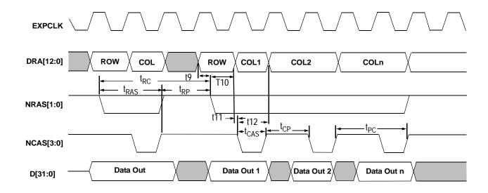
Figure 18. DRAM Write Cycles at 13 MHz and 18 MHz
