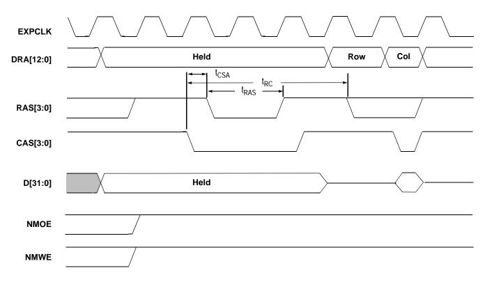
Figure 22. DRAM CAS Before RAS Refresh Cycle at 13 MHz and 18 MHz
