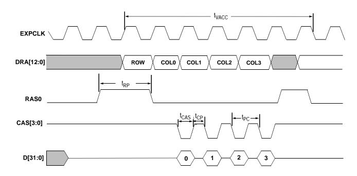
Figure 20. Video Quad Word Read from DRAM at 13 MHz and 18 MHz
