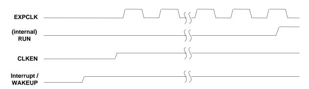
Figure 5. CLKEN Timing Entering the Standby State
