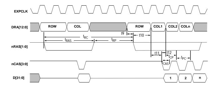
Figure 17. DRAM Read Cycles at 36 MHz
