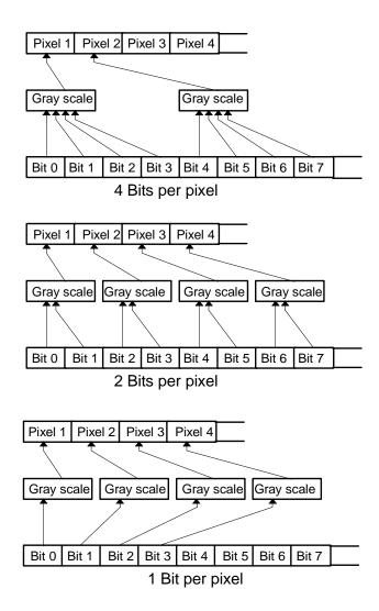
Figure 11. Video Buffer Mapping
