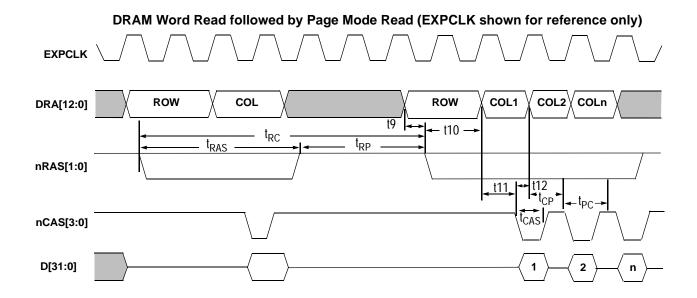
Figure 16. DRAM Read Cycles at 13 MHz and 18.432 MHz
