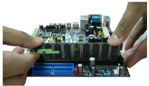
• Firmly insert the DIMM into the socket until the retaining clips snap back in place and the DIMM is properly seated.
