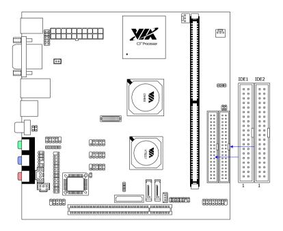
If two drives are connected to a single cable, the jumper on the second drive must be set to slave mode. Refer to the drive documentation supplied by the vendor for the jumper settings. Both IDE1 and IDE2 have a  $20^{th}$  pin included. The  $20^{th}$  pin was added to provide extra voltage to power 40-pin Disk-on Modules (DOM). See voltage selector: J1 on page 38 and 40. You must use IDE cables that do not block the  $20^{th}$  pin.
