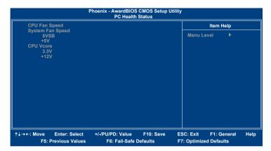
The PC Health Status displays the current status of all of the monitored hardware devices/components such as CPU voltages, temperatures and fan speeds.
