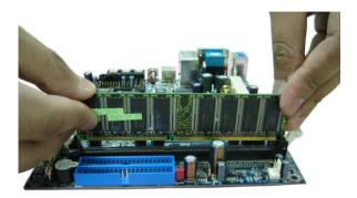
• Align a DIMM on the socket such that the notch on the DIMM matches the break on the socket.
