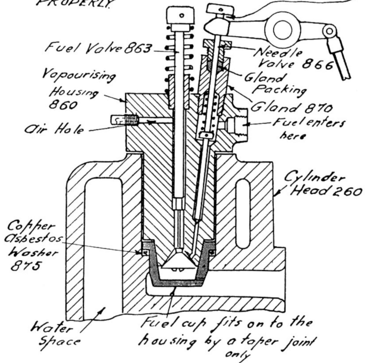
The small holes in the fuel cup must always point towards the piston.
