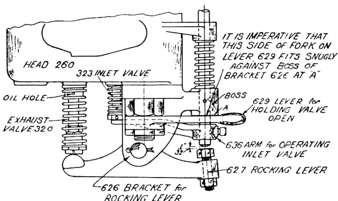
**To Adjust Arm 636 to Operate Inlet Valve** (see above illustration).-Turn the Engine slowly in the usual running direction, until the Exhaust Valve just closes (i.e., when the piston is at the head end of the Engine), lift lever 636, and slide arm along pushrod till it just touches the end of the inlet valve, then tighten the square-headed set screw on arm 636.
